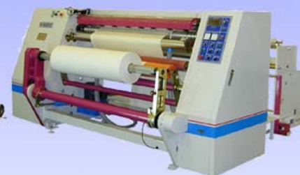
HY-SDT Center-Surface Rewinder Rewind O.D :600mm Paper Core: 3"
