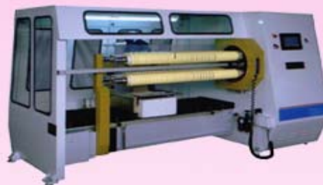
HY-FQ Single Blade 4 Shafts Exchange Auto Cutter Cutting O.D. : 180mm
