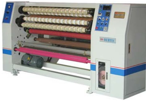
HY-BA 4 Shafts Exchange Slitter (Razor Blade) For: OPP Packaging, Stationery Tapes...etc. Min. Slitting Width: 12mm Max. Rewind OD: 150mm
