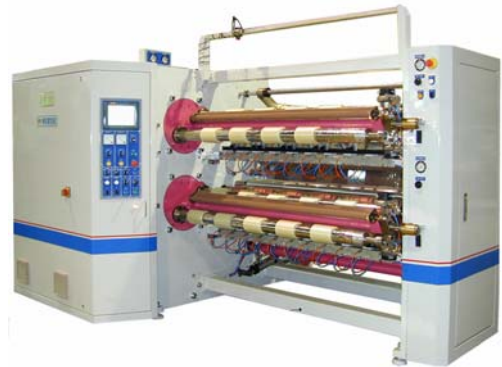
HY-BAL 4 Shafts Exchange Slitter For: OPP Packaging, PET Tapes...etc. Min. Slitting Width: 80 mm Max. Rewind OD: 180mm Special Device: Surface Type Rewind Lay On Roller To Erase Air Bubble in Log Roll.
