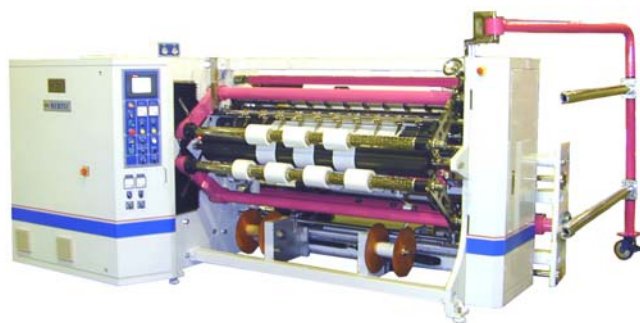
HY-ESF 2 Shafts Center Rewind, For Slitting PET, Reflector, Release Film, Diffused Film & BEF...etc. Width: 1.0M/1.3M/1.6M Max. Unwind O.D: 800mm Min. Slitting Width: 50mm Max. Rewind O.D: 400 & 600mm
