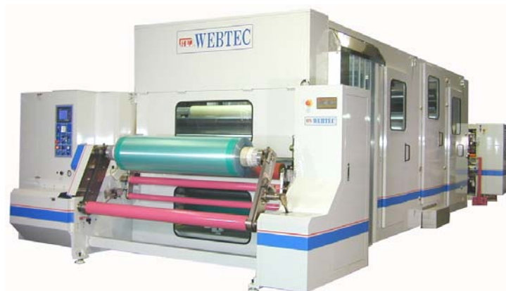
HY-SDLF-I 1 shaft center type winding, suitable for inspecting & laminating BEF, DBEF, TDF...etc. (Available for two layers lamination and 1 or 2 or 3 stages inspection) Width: 1.0M/1.3M/1.6M Max. Unwind & Rewind O.D: 900mm Protection film Rewind O.D : 500mm
