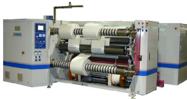
HY-TEF 2 Shafts Center Rewind, For Slitting Reflector, BEF & PET...etc. Width: 1.0M/1.3M/1.6M/2.0M Max. Unwind O.D: 800mm Min. Slitting Width: 150mm Max. Rewind O.D: 600mm
